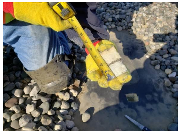
6. View of the roof core from the smaller south building addition where two layers of 1.5" foam exist.
