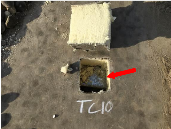
15. Photo of Test Cut #10. Insulation found dry to touch.
