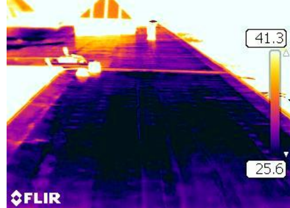
4. Image 4. A 4 th look at a smooth 2008 area roof. No localized heat images that would be suspect of representing wet insulation.
