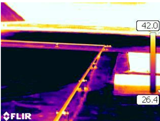
5. Image 5. One more smooth roof. No localized heat images that would be suspect of representing wet insulation. Conduits visible.
