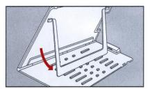
3. Lift inside support to one of six positions for desired reading angle. Adjust to avoid glare and shadows. Snap into place.
